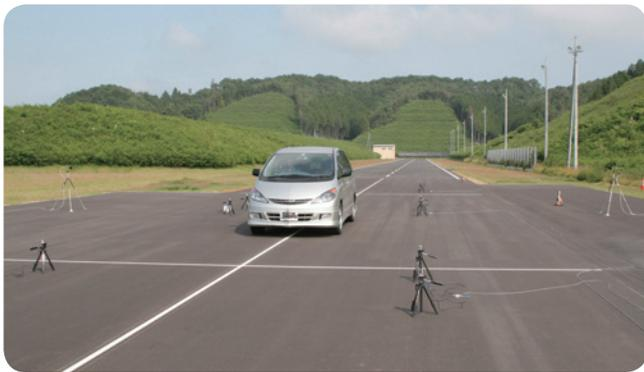
A vehicle undergoing the R51 acceleration test.
